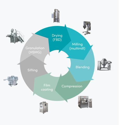
Figure 1. Manufacturing flow of the fixed-dose combination drug product
